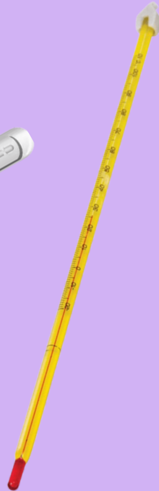
LABORATORY THERMOMETER measure the temperature of liquids (-10 to 110°C)
